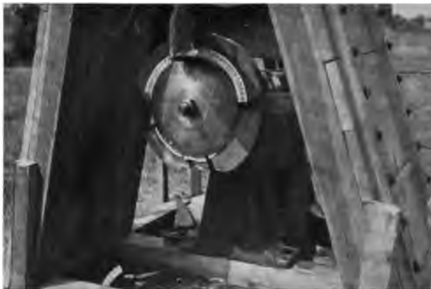
Fig. 2. Test of Tapered Flanges, showing that pieces may break and fly from portion of wheel outside flanges.
